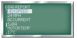
12. MOTOR CURRENT: displayed as 'AC CURRENT', the next line displays the AC current in Amps.
