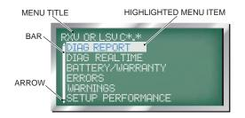
To access the different diagnostic functions, use the five control buttons to scroll through the menus.
