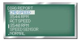
MOTOR ACTUAL SPEED: displayed as 'ACTSPEED', the next line displays the actual motor speed in RPMs.
