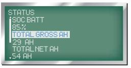
48. TOTAL NET AMP-HOURS: displayed as 'TOTAL NET AH', this is the total net Amp-Hours used for the life of the vehicle.
