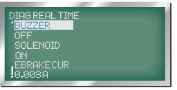
41. SOLENOID: displayed as 'SOLENOID', the next line displays the solenoid state as 'ON' or 'OFF'.
