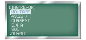
CALCULATED BATTERY CURRENT: displayed as 'CURRENT', the next line displays calculated current as 'HIGH', 'LOW' or the actual number in DC Amps.
