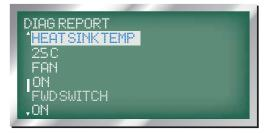
FAN function is displayed as "FAN", the next line displays whether or not the controller cooling fan is on or off.
