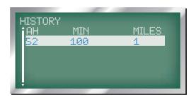
53. TOTAL RUN TIME ON VEHICLE IN MINUTES: displayed as 'MIN', this is the total run time on vehicle in minutes since the the last recorded charge cycle.
