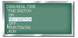
39. RUN TOW SWITCH POSITION: displayed as 'RUN TOW SW', the next line displays the position of the run/tow switch as 'RUN' or 'TOW'.
