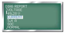
STATE OF CHARGE: displayed as 'SOC', the next line displays the state of charge for the battery pack as 'HIGH', 'NORMAL' or 'LOW BATT'.
