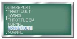
BRAKE SWITCH POSITION: displayed as 'BRAKE SW' the next line displays the switch voltage as 'NOR-MAL' or 'ABNORMAL'.
