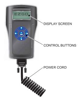
With the vehicle key switch in the 'OFF' position, the hand held diagnostic unit is connected to the vehicle by plugging the power cord connector into the receptacle (CAN) located under the vehicle cup holder. Turn the key switch on to power up the hand held. If the hand held shows 'no connection' or a blank screen, check the cord and the CAN connections and wiring.
