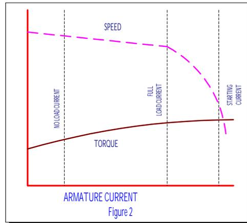
In the separately excited motor, the motor is operated as a fixed field shunt motor in the normal running range. However, when additional torque is required, for example, to climb non-level terrain, such as ramps and the like, the field current is increased to provide the higher level of torque. In most cases, the armature to field ampere turn ratio can be very similar to that of a comparable size series motor (Figure 3.)
