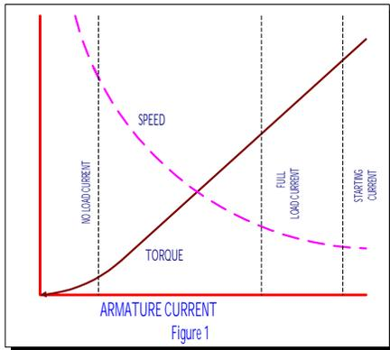
As shown in the typical performance curves of Figure 1, the high torque at low speed characteristic of the series motor is evident.
