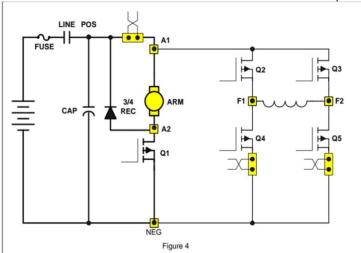
By energizing the transistors in pairs, current can be made to flow in either direction in the field. The field and armature control circuits typically operate at 12KHZ to 15KHZ, a frequency range normally above human hearing. This high frequency, coupled with the elimination of directional contactors, provides for very quiet vehicle operation.
