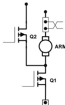
Slow down is accomplished when reversing direction by providing a small amount of retarding torque for deceleration. If the vehicle is moving, and the directional lever is moved from one direction to the other, the regen signal is initiated. Once the regen signal has been initiated, the field current is increased. Armature current is regulated to the regen current limit
