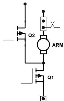
Slow down is accomplished when reversing direction by providing a small amount of retarding torque for deceleration. If the vehicle is moving, and the directional lever is moved from one direction to the other, the regen signal is initiated. Once the regen signal has been initiated, the field current is increased. Armature current is regulated to the regen current limit
