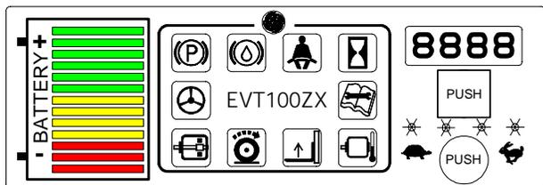
The Interactive Custom Dash Display allows the operator to select the best vehicle performance for changing factory (task) conditions. There are four (4) "operator interaction modes" that can be selected by depressing a push-button on the dash display.
