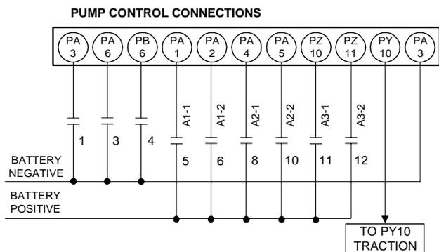
**Section 5.4.4 Typical Brush Wear Sensor Connections For Pump Control**
