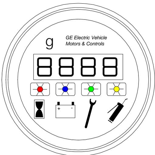
The GE Standard Dash Display is a four segment Light Emitting Diode (LED) instrument that displays the GE LX, ZX, and SX Status Codes, Hourmeter Readings, Battery Discharge Indication, and Maintenance Required Code. The four LED's above the symbols indicate the active readout mode.
