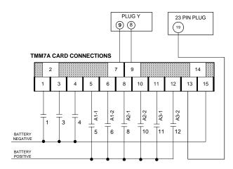
**Section 5.4.2 Typical Brush Wear Sensor Connections**
