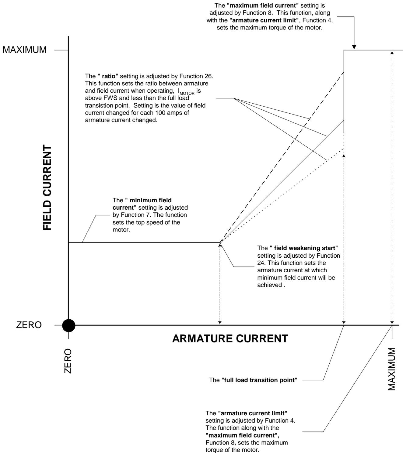
**Section 6.6 Setup Functions for Hydraulic Pump Control**
