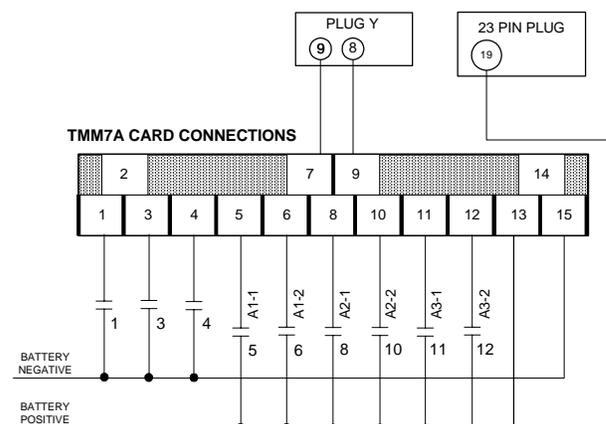
**Section 5.4.2 Typical Brush Wear Sensor Connections**
