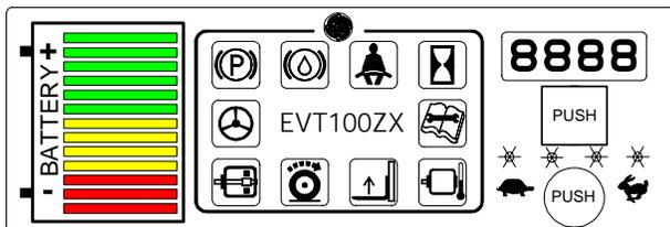
The Interactive Custom Dash Display allows the operator to select the best vehicle performance for changing factory (task) conditions. There are four (4) "operator interaction modes" that can be selected by depressing a push-button on the dash display.
