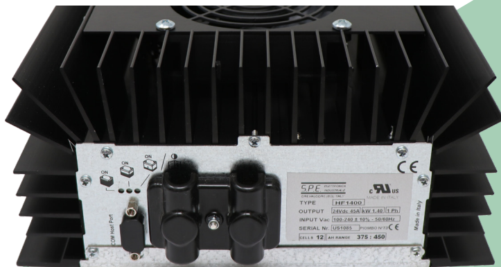
Multicolor LED indicator for faults and charging status
