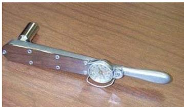
Calibrated torque wrench for hardware installation
