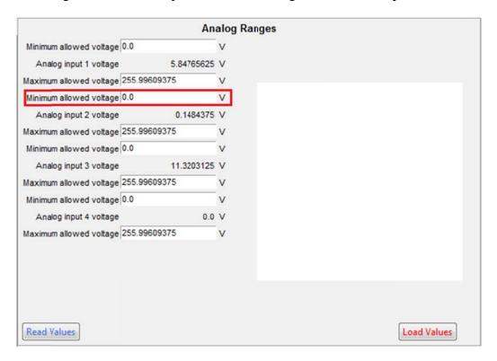
The setting highlighted above is going to be changed (in this case, the minimum allowed voltage of AU2) from 0 to 5v. To do this, first click inside of the appropriate text box, and delete the contents.
