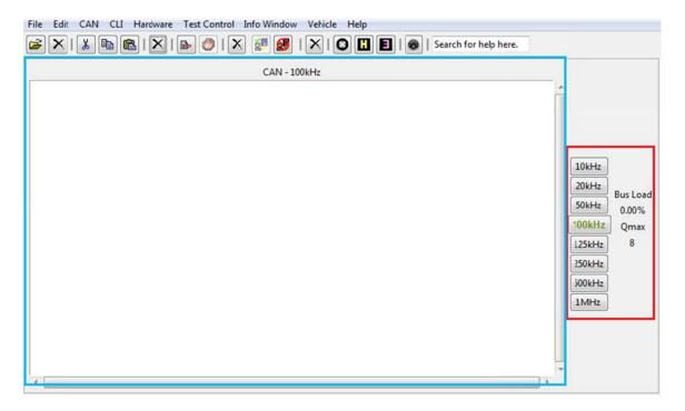
The different baud options can be seen inside the red box. There is currently an incorrect baud of 100 kHz rate selected. This is visible because the CAN window (seen in the blue box) is empty, and the software is unresponsive. If an incorrect baud rate is selected then the CAN window remains blank.
