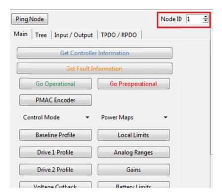
By clicking the small arrows seen above, I can cycle through different node ID numbers. There is no alert system or notification. As soon as the number changes; helper commands will be sent to that node.
