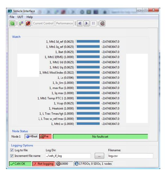
This window will update in real-time with settings and information about the motor controller setup. Information displayed depends on the TPDO setup of the motor controller.
