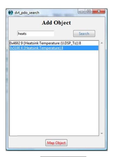
Write PDO Finally, select the button, close and re-open the helper to ensure the changes have happened.
