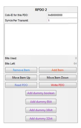
Each PDO must have a unique Cob-ID which denotes the priority of the associated PDO, the lower the number; the higher the priority of the PDO.
