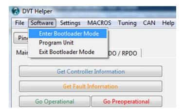
While in bootloader mode; the motor controller will be unresponsive to commands, and will display errors or timeout when changes are attempted to anything aside from software.
