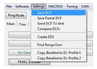
Selecting "Save DCF" will save the current configuration inside the controller to wherever the user wants. Changing DCF however is done through the "Send DCF to Unit" option found here:
