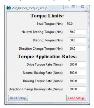
The peak torque showed on this trace is the actual torque configured (See local limits window) in Nm and its dependent on the motor manufacturer. The values showed below peak torque are all related to the peak torque and the percentages set in the baseline profile. The torque limits are in Nm and rates are Nm/s.
