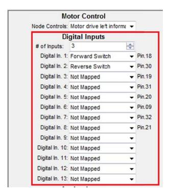
To begin with, the "'# of inputs" setting has to be set exactly. For example, if the number is set to four, but there are five inputs configured; the helper will stop reading after input number four.
