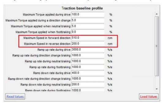
The setting highlighted above is going to be changed (in this case, the maximum forward rpm) to 600 and the reverse to 450. To do this, first click inside of the appropriate text box, and delete the contents.
