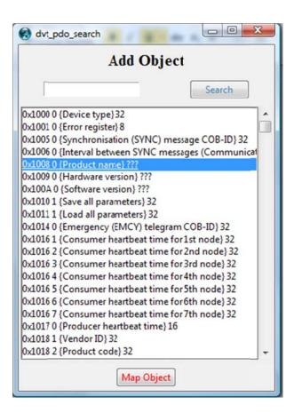
RPDO2 in this scenario is going to be given the "Battery Voltage" and "Vehicle Speed". To do this, the procedure is the same as seen in the TPDO section of this guide:
