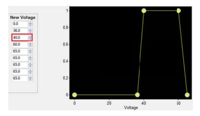
Alternatively, new values can be entered into the boxes manually through the keyboard. The same customisation can be applied to the level of torque that is cut back in the same way. This is seen under the "New cutback" gain.
