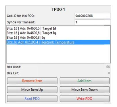
Note: When adding objects into a PDO, ensure that there are adequate bits left for the desired objects.
