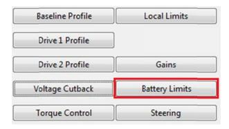
Selecting the button will bring up a menu on its' right side containing the voltage settings for the controller. To change the under voltage limit (the minimum voltage that can be set without the line contactor opening) from 21.0V to 30V, the process is as follows:
