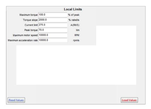
From this menu, the user can access the torque and current settings of the motor attached to the system. To change the current limit (the minimum voltage that can be set without the line contactor opening) from 275A to 280A, the process is as follows:
