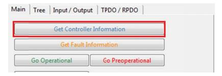
Selecting this button will cause a new window to open, which will fill with information on the controller:
