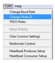
This will open a small window inside the helper in which the user can set the new CAN ID, in this scenario the ID will be set to 2.
