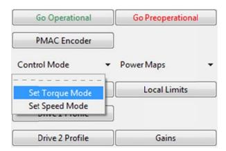
When switching the control mode, DVT will first be automatically put into pre-op.
