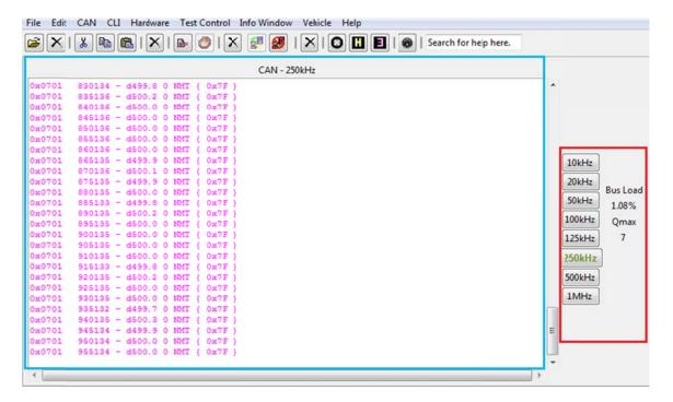
If correct baud is selected then CANBus transmissions will be seen scrolling in the CAN window. The DVT is now ready to perform operations
