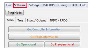
Selecting this tap will open a small drop down menu, to begin the process of installing a new DLD; first select the "Enter Bootloader Mode" option found here:
