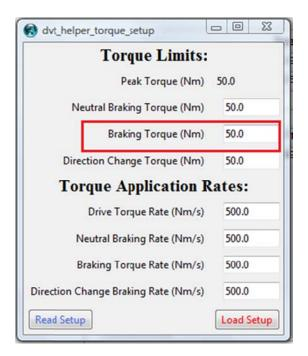
The braking torque (highlighted above) will be changed from 3.5Nm to 20Nm as an example of how to change a setting. To do this, first click inside of the appropriate text box, and delete the contents.
