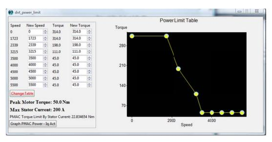
From this table/graph, the speed and torque settings can both be changed through the same means used in the *Voltage Cutback* section of this manual.
