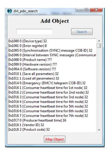
Selecting the search button or pressing any key will cause the window to fill with objects.
