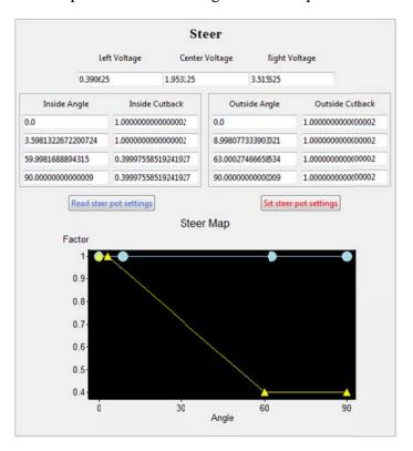
From this menu, voltages corresponding to fully left (-90 degrees), straight ahead (0 degrees) and fully right (90 degrees) are accessible. The corresponding values are used by the Gen 4 to calculate the steering angle based on the analogue voltages from the steering potentiometer.
