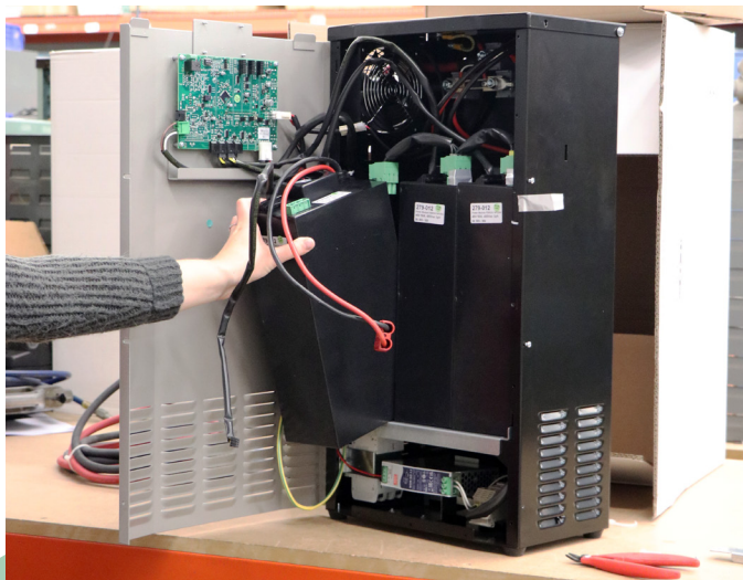
Photo is of a GREEN6 , the GREENX will have 5–6 modules.
