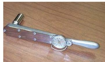
Calibrated torque wrench for hardware installation
