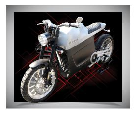
The Luna is powered by an efficient 55-horsepower PMAC electric motor and Sevcon Gen 4 motor controller, and fed by a custom 11.8kWh lithium battery pack. Re-energizing duties of the Luna are handled by a 3.3kW onboard charger, along with a regenerative braking system.
