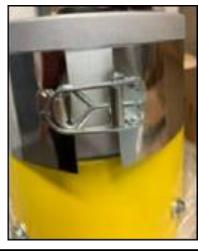
**3.** Loosen the 2 (10MM) bolts as seen below. These bolts are clamping the spade terminals that are attached to the brush.
