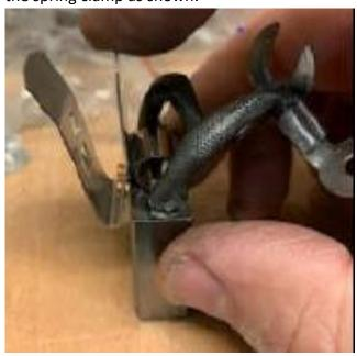
**8.** Gently slide the combination of spring and brush into the location from which it was removed.
