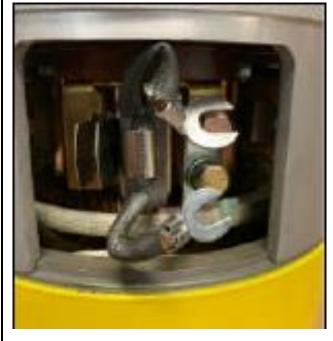
**9.** Slide the terminals under the bolts making sure that the terminals are under the supplied washers.
