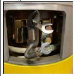
**6.** Using pliers, remove the spring clip by squeezing the clip as shown.
