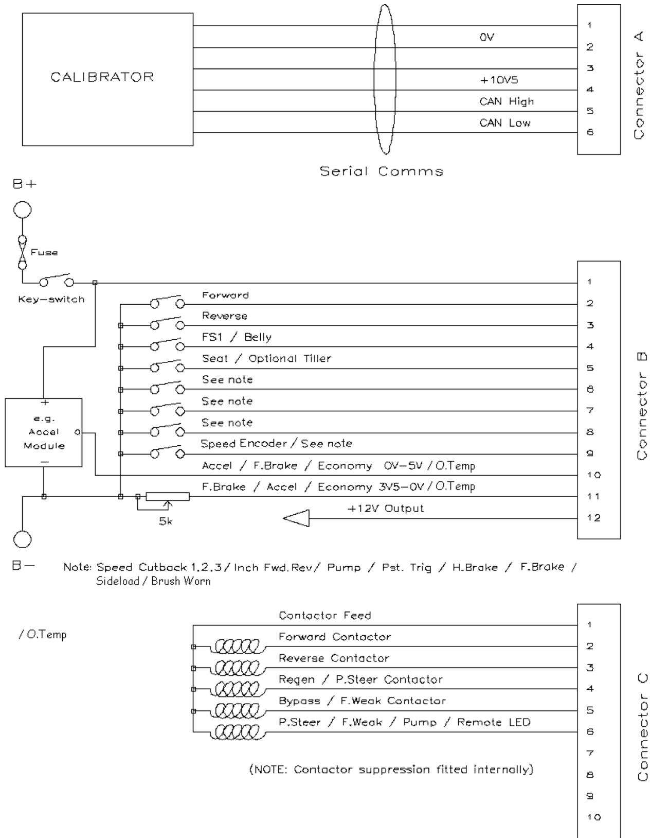
**Figure 3 Light Wiring - High I/O Logic**
