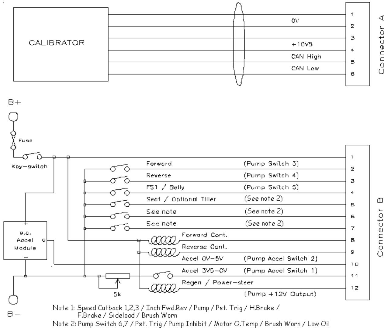
**Figure 2 Light Wiring - Medium I/O Logic**
