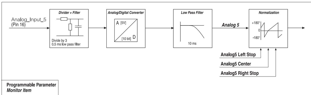
**Fig. 10** Position Feedback Device "0" signal flow (Analog 5 shown; Analog 6 is similar).
