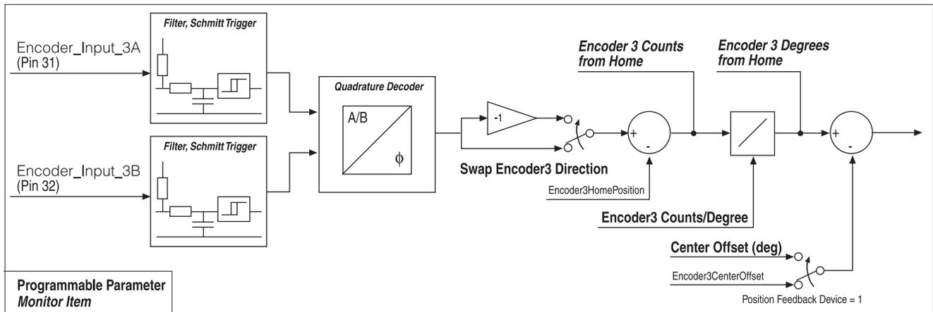
Fig. 11 Position Feedback Device “1” signal flow (Encoder 3 shown; Encoder 4 is similar).
