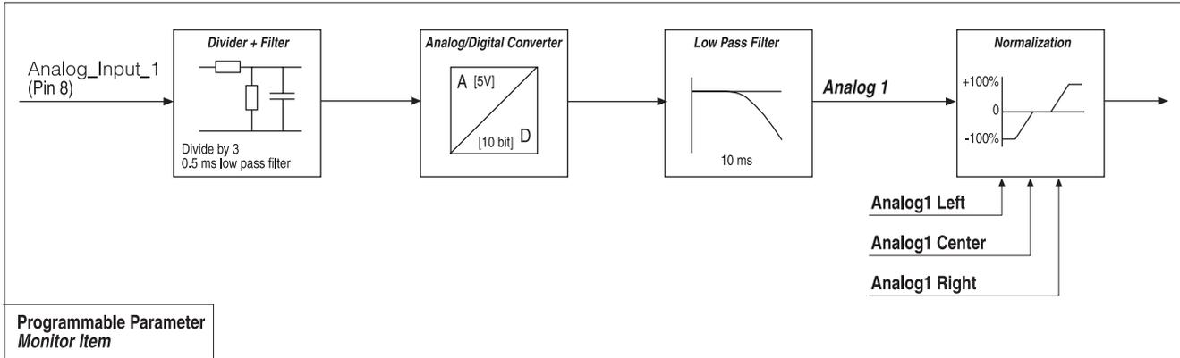
**Fig. 4** Command Input Device "0" signal flow (Analog 1 shown; Analog 3 is similar).
