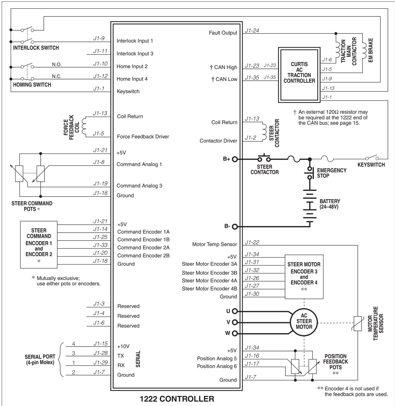
Fig. 3a Wiring diagram, Curtis 1222 electric steering controller.
