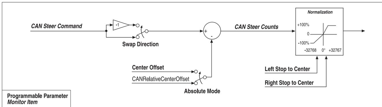
**Fig. 8** Command Input Device “4” signal flow.
