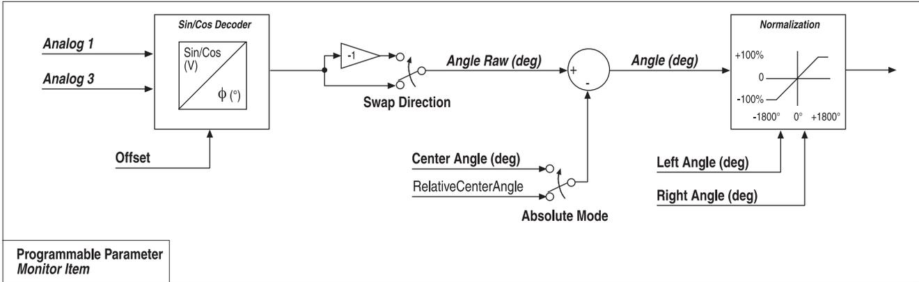
**Fig. 6** *Command Input Device "2" signal flow.*
