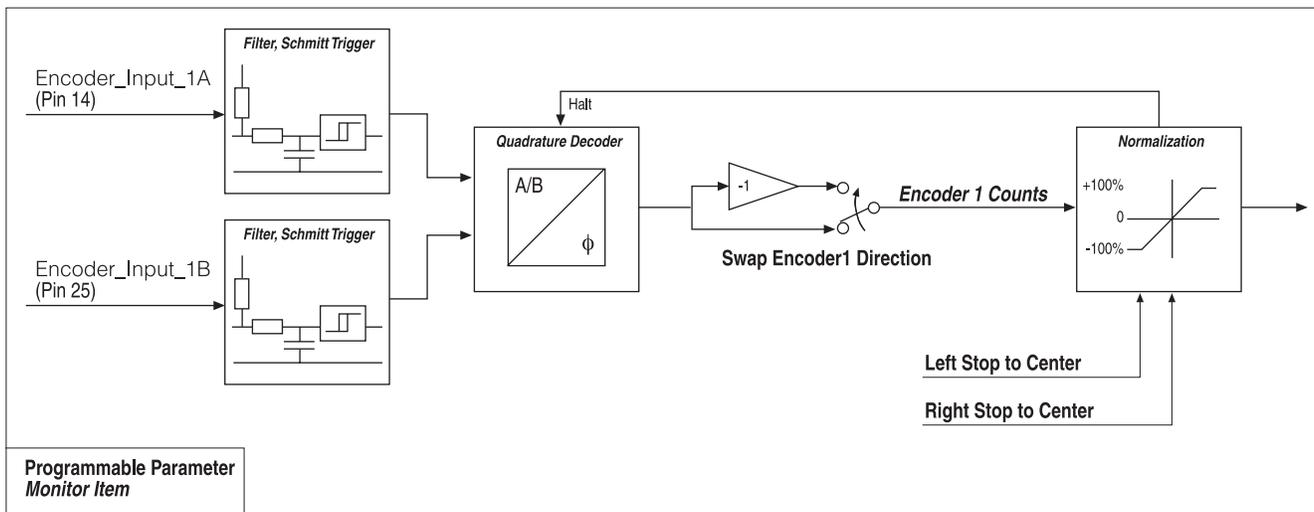
Fig. 5 Command Input Device “1” signal flow (Encoder 1 shown; Encoder 2 is similar).
