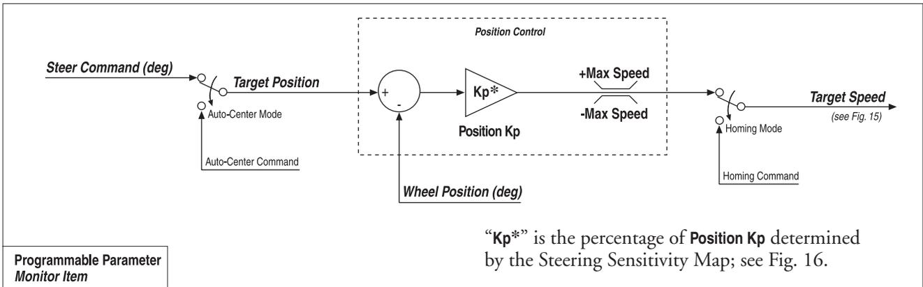
Fig. 14 Position Control signal flow.
