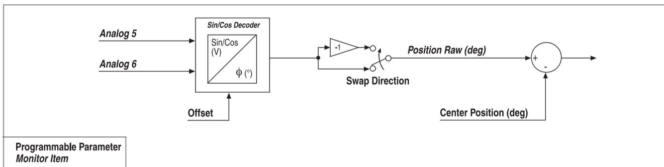
**Fig. 12** Position Feedback Input Device "2" signal flow.
