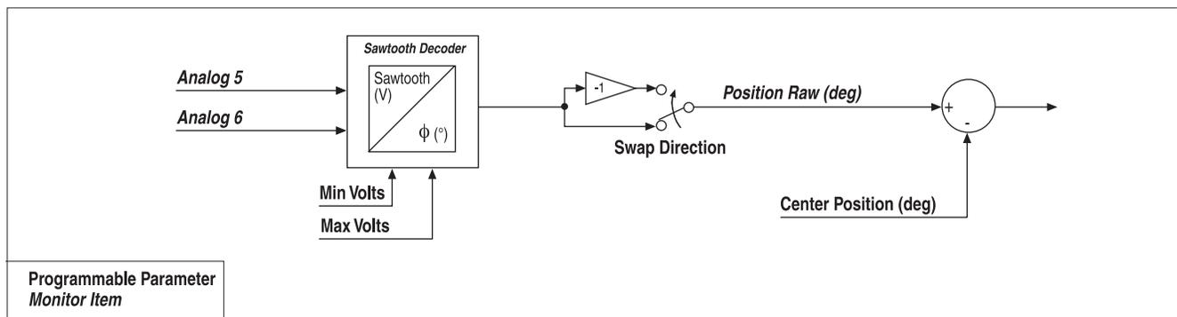
Fig. 13 Position Feedback Input Device "3" signal flow.
