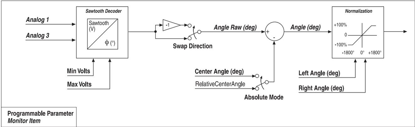
**Fig. 7** Command Input Device "3" signal flow.
