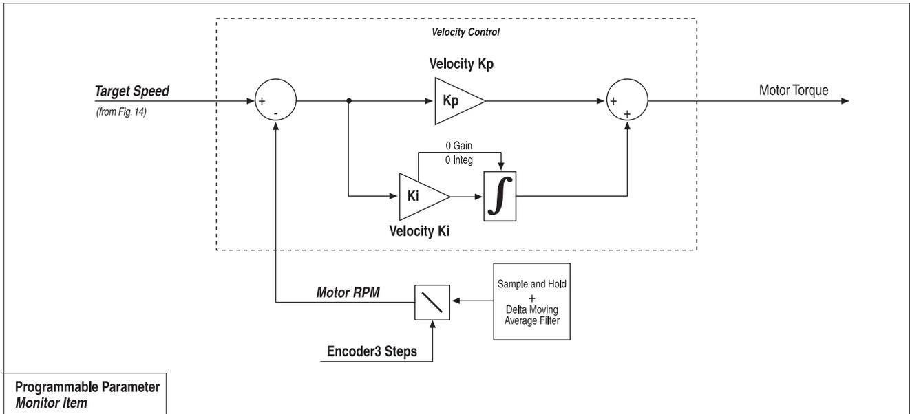
Fig. 15 Velocity Control signal flow.
