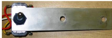
7.) Install the contactor bracket onto the floor pan in front of the control. There are holes in the floor pan in which the bracket can be mounted with nuts and bolts (**Figure 11**).
