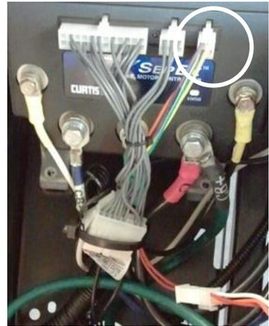
**7.** Remove the solenoid environmental protection cover.
