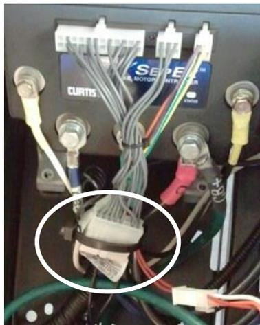
**6.** Insert the 4 pin original wire harness plug into the new controller.
