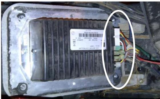
3. Carefully unplug all connections to the factory controller and remove the three – 13mm bolts securing the four large diameter wires. Save these bolts they will be reused when installing the new controller.
