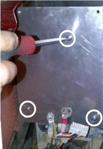
2. Using the original controllers mounting bolts and holes mount the conversion plate to the vehicle heatsink.
