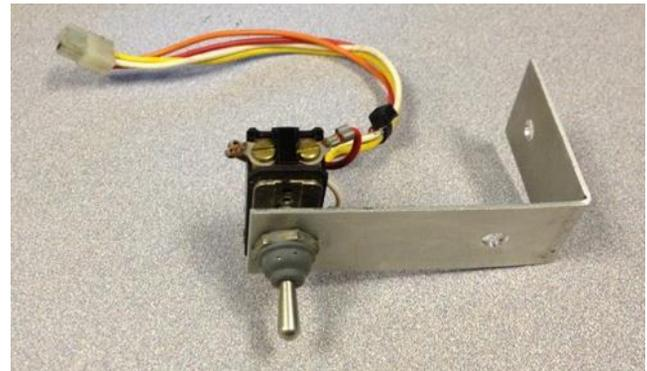
**13.** Re-install the tow/run switch in the new mount provided using the original hardware.
