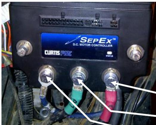
1. Using the three 13mm bolts retained when the original controller was removed, securely fasten the four large diameter wires to the new controller.
