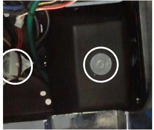
**12.** Remove the tow/run switch from the original controllers environmental cover.
