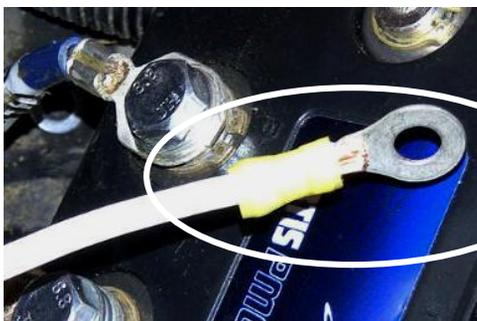
2. The new controller uses ring terminals instead of faston connectors for the field connections. Using a wire crimper and the two ring terminals (included) cut and re-crimp the black and white 10awg wires coming from the motor.
