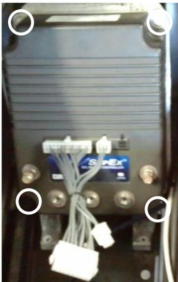
4. Using the four M6 bolts, washers, and lock washers (included) securely mount the new controller to the adapter plate previously installed.
