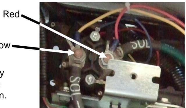
**11.** Plug the two wire- four pin walk-away harness connector to the two wire- four pin conversion harness connector then re-install solenoid cover using original hardware.
