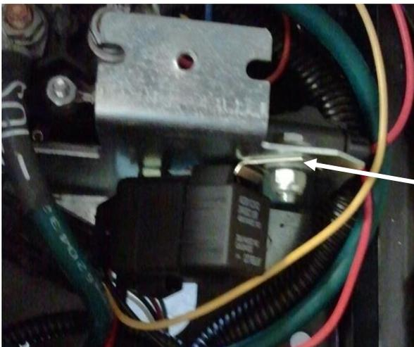
**9.** Using the supplied M5x20mm bolt, washers, lock washer, and nut attach the walk-away relay and fuse to the solenoid cover mounting tab as shown.
