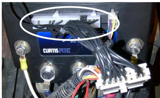
4. Insert the conversion harness into the new controller's 6 and 24 pin connectors.
