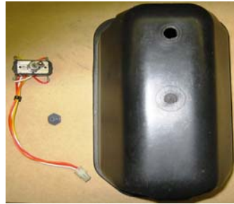
Tow/Run switch, mounting nut, and cover after disassembly
