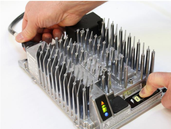
2. While reconnecting AC input, press and hold the Select Charge Profile Button. Hold the button (approximately 10 seconds) through the light check function until Error Indicator is on (in amber) and Battery Charging Indicator (in green) starts flashing.
