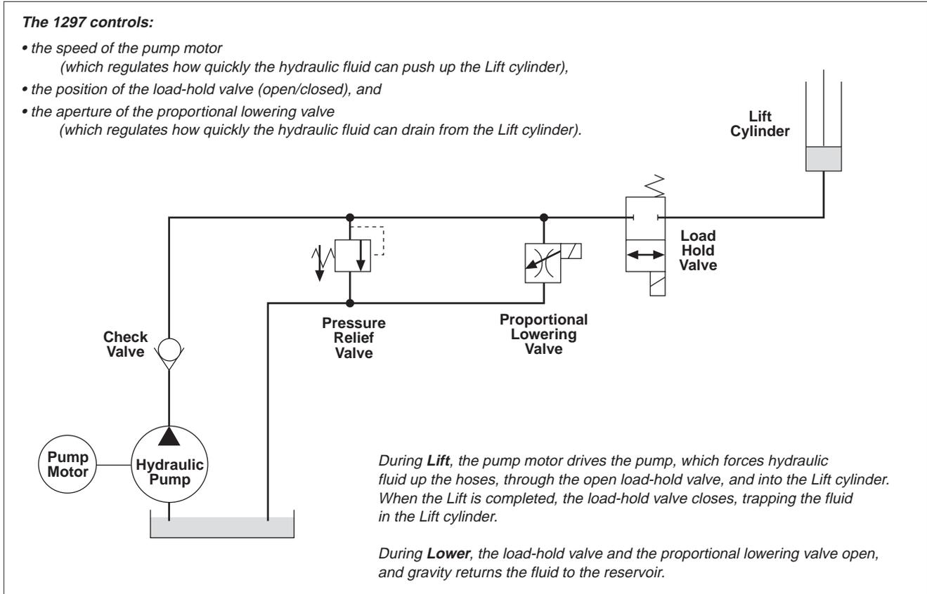
**Fig. 20** Hydraulic system diagram.
