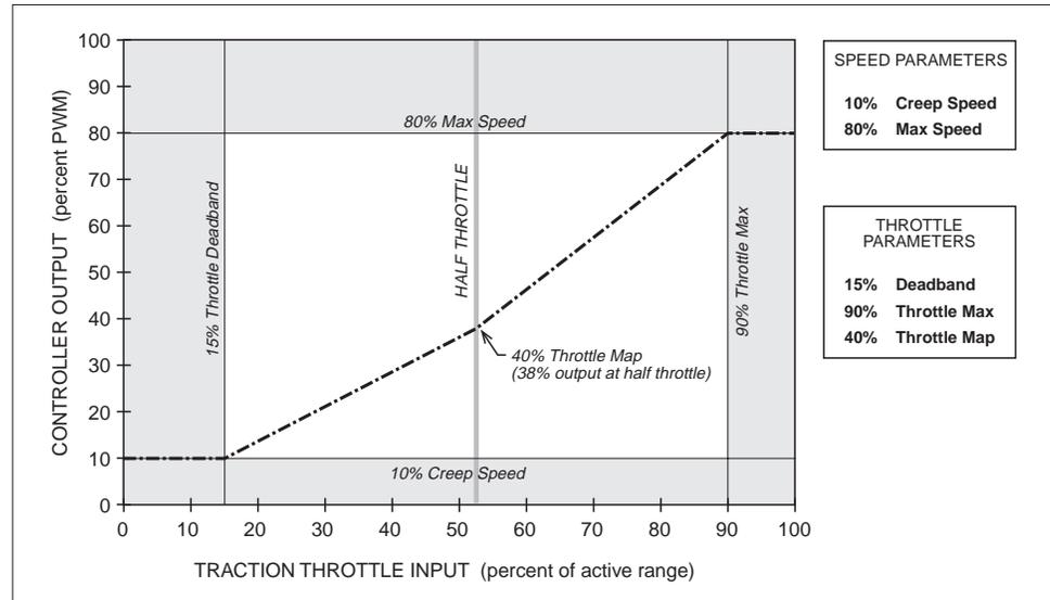
range. These four parameters, together with the throttle map, determine the controller's output response to throttle demand.
