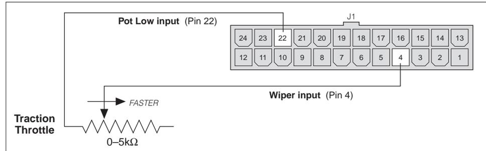
Broken wire protection is provided by the controller sensing the current flow from the wiper input (Pin 4) through the potentiometer and into the Pot Low pin (Pin 22). If the Pot Low input current falls below 0.65 mA or its voltage below 0.06 V, a throttle fault is generated and the throttle request is zeroed. NOTE: The Pot Low pin must not be tied to ground (B-).
