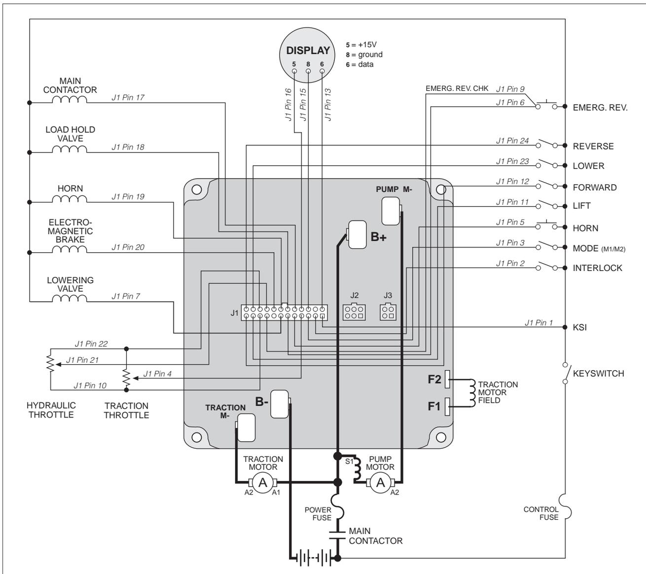
**Fig. 3** Standard wiring configuration, Curtis PMC 1297 controller, with no tiller multiplexer connected to the 6-pin connector.
