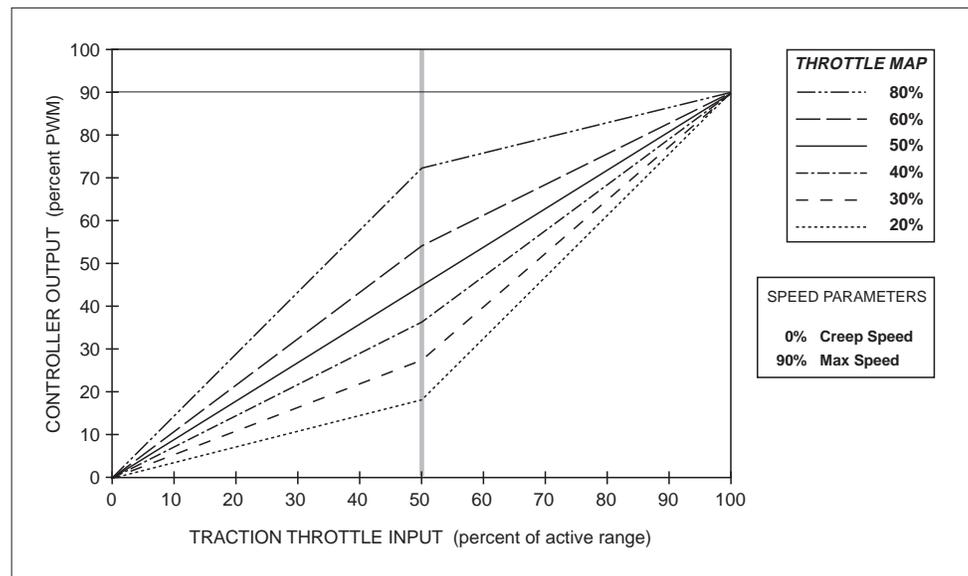
The throttle map operates within the window established by the Creep Speed, Max Speed, Throttle Deadband, and Throttle Max parameters, as shown in Figure 18. Creep Speed and Max Speed define the controller's output range, while Throttle Deadband and Throttle Max define the throttle's active
