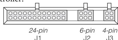
The 24-pin connector (J1) provides the logic control connections for the contactor drivers and switches that are wired directly to the vehicle. The mating connector is a 24-pin Molex Mini-Fit Jr. connector part number 39-01-2245 using type 5556 terminals.
