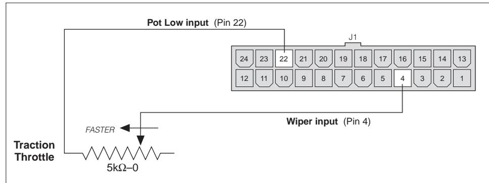
Broken wire protection is provided by the controller sensing the current flow from the wiper input (Pin 4) through the potentiometer and into the Pot Low pin (Pin 22). If the Pot Low input current falls below 0.65 mA or its voltage below 0.06 V, a throttle fault is generated and the throttle request is zeroed. NOTE: The Pot Low pin must not be tied to ground (B-).
