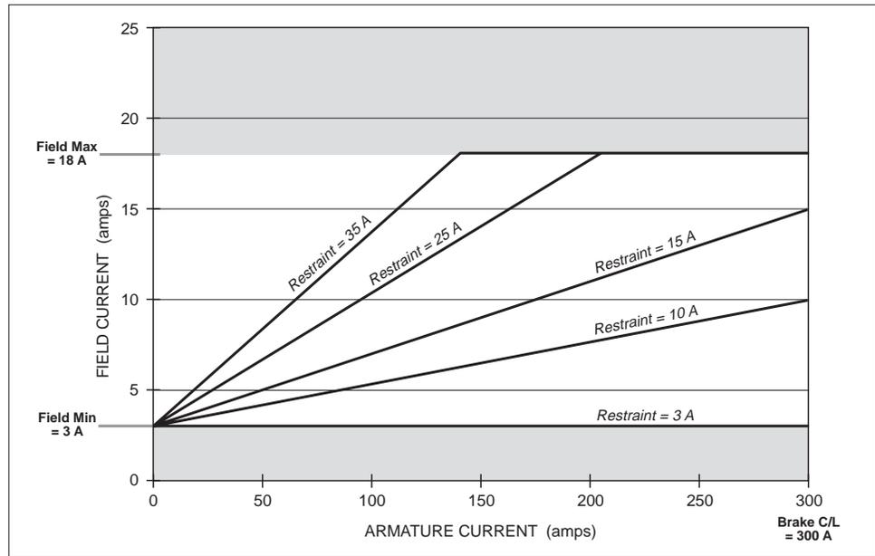
slower the vehicle will creep down ramps. This creeping speed depends on the restraint setting, the steepness of the ramp, and the vehicle load weight. The restraint feature can never hold a vehicle perfectly stationary on a ramp and is not intended to replace a mechanical or electromagnetic brake for this purpose.
