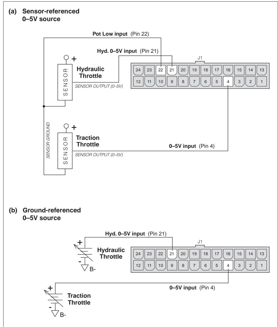
Also, the controller recognizes the voltage between the wiper input and B- as the applied throttle voltage and not the voltage from the voltage source relative to the Pot Low input.
