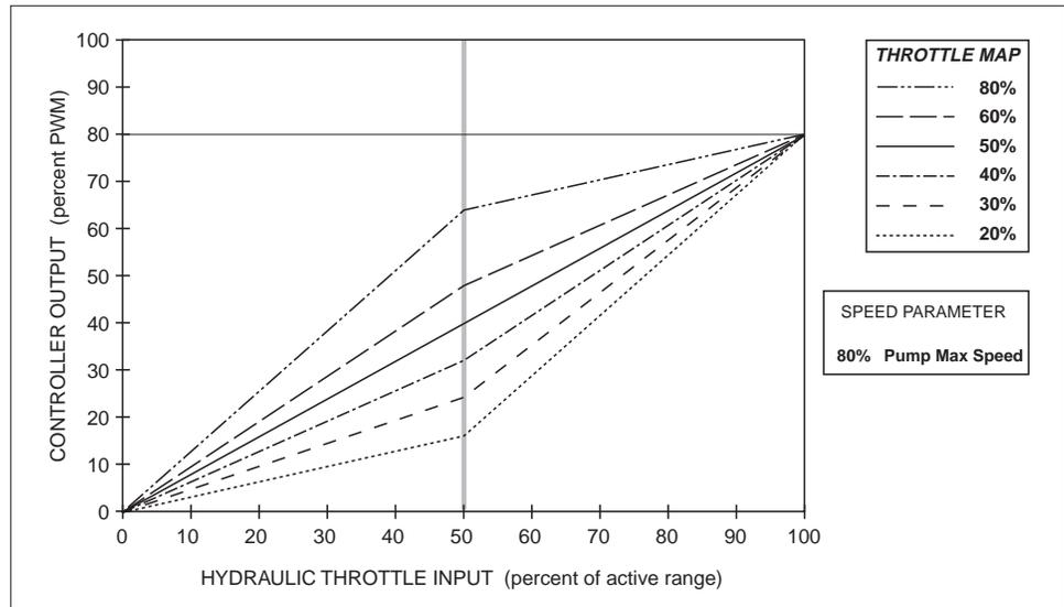
to increase as soon as the throttle is rotated out of its normal neutral range (deadband). Controller output will continue to increase, following the curve defined by the throttle map setting, as the throttle input increases and will reach maximum output when the throttle input enters the upper deadband (crosses the Throttle Max threshold).
