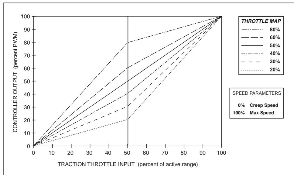
Raising the creep speed parameter or lowering the maximum speed parameter limits the controller's output range, as shown in Figures 16 and 17. Controller output is always a percentage of the range defined by the speed parameters (the range between the creep speed and maximum speed settings).
