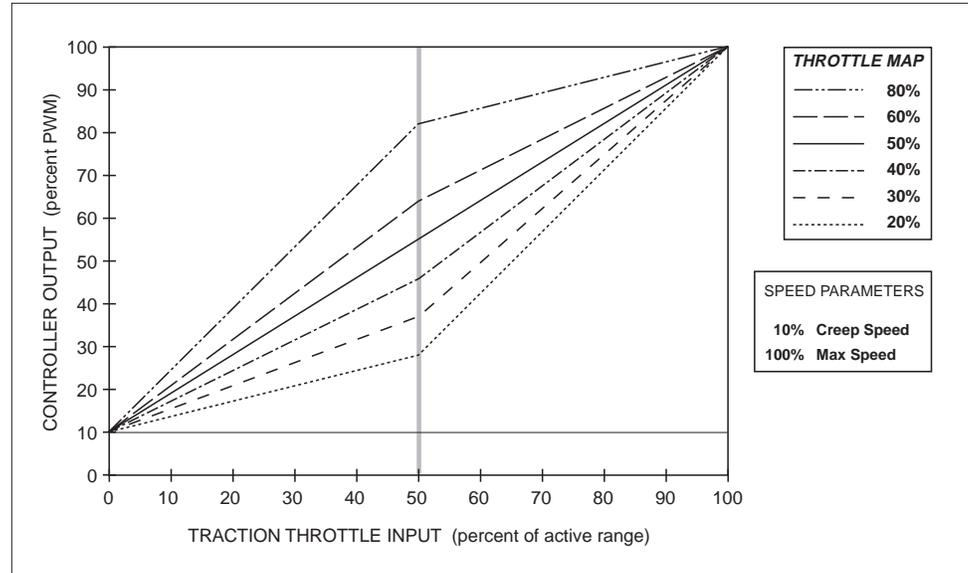
In Figure 17, the maximum speed is decreased to 90% and the creep speed is left at 0%; again, the controller output range is 90%. With these speed settings, a 50% throttle map will result in 45% output at half throttle.
