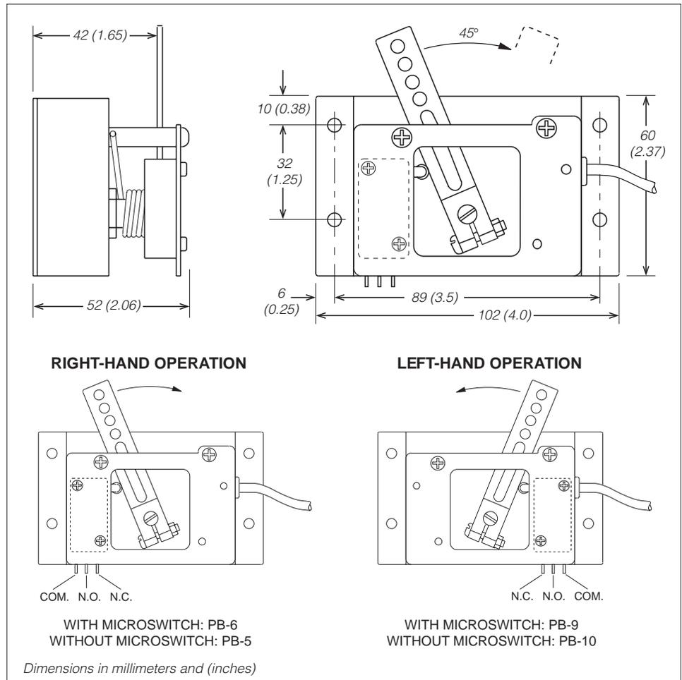
**Fig. B-3** Mounting dimensions, Curtis PMC footpedal FP-2.
