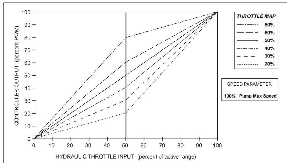
Reducing the maximum pump speed will limit the controller's output range. Throttle map profiles with the maximum pump speed reduced from 100% to 80% are shown in Figure 245. The throttle map is always a percentage of the controller's output range. So, in these examples, the throttle map is a percentage of the 0–80% output range; a 40% throttle map setting will give 32% output at half throttle (40% of 80% = 32%). Controller output will begin
