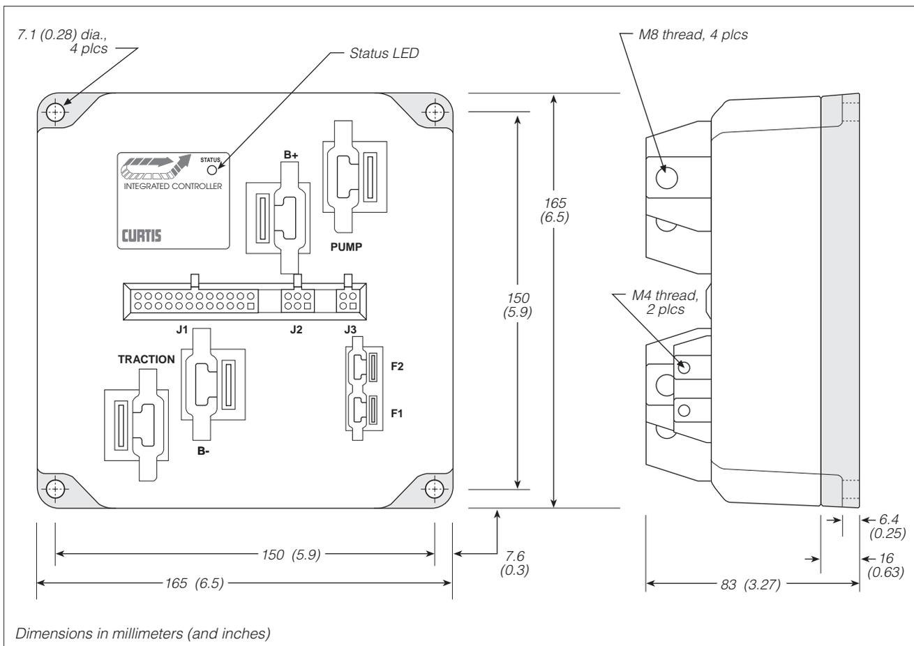
**Fig. 2** Mounting dimensions, Curtis PMC 1297 controller.
