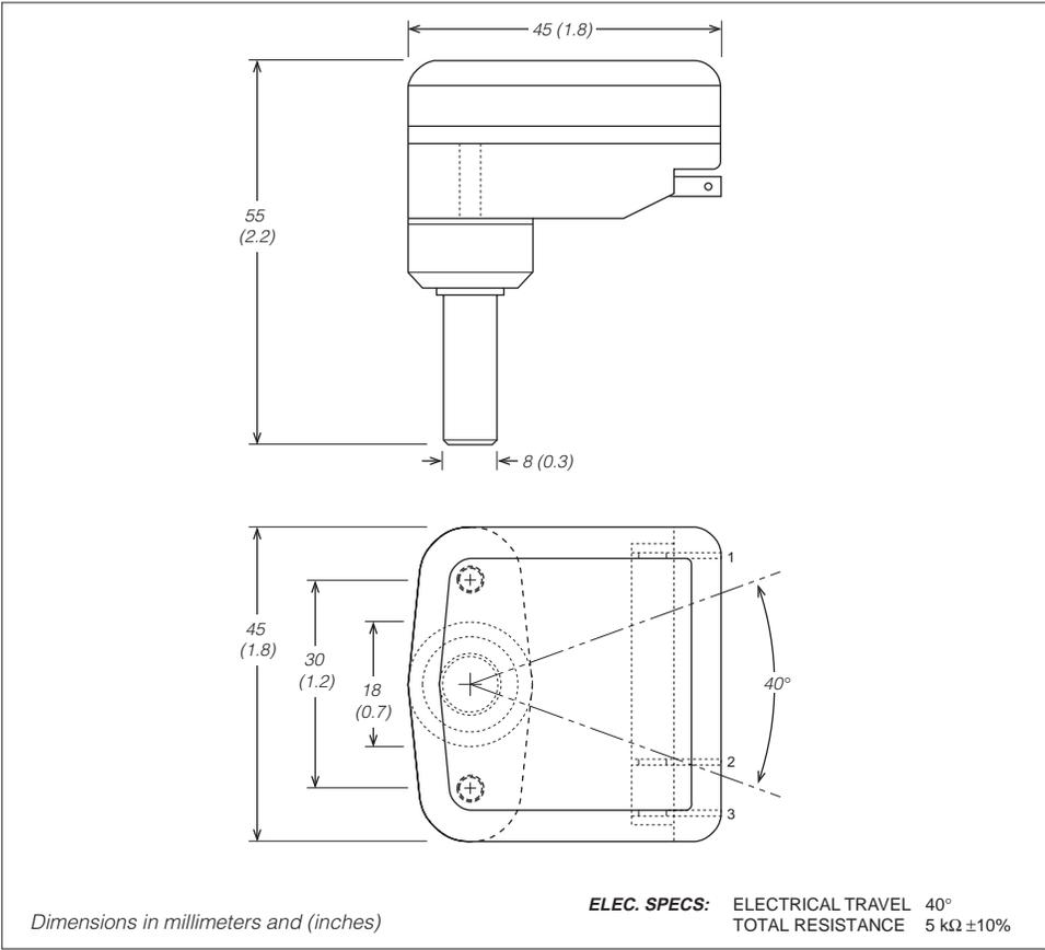
**Fig. B-5** *Mounting dimensions, Curtis electronic speed control device (ET series).*
