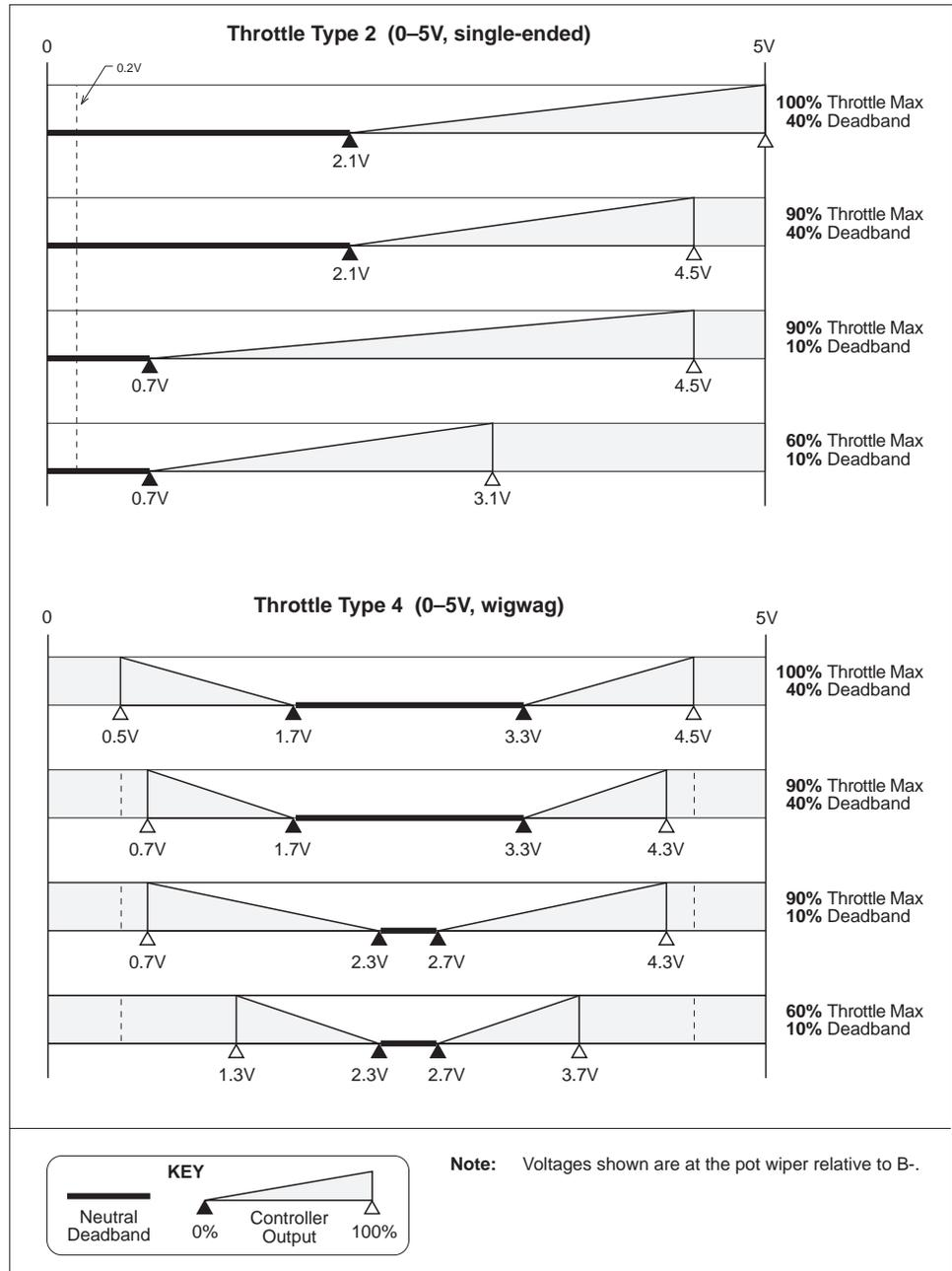
The programmer displays hydraulic Throttle Max as a percentage of the throttle's active voltage range. The nominal voltage range depends on the throttle type selected. See Table 1 (page 12) for the characteristics of your selected throttle type. The hydraulic Throttle Max parameter can be adjusted from 100% to 60%, in 1% increments.
