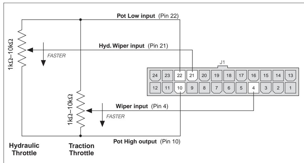
When a 3-wire pot is used and the Pot Low Check parameter (see Section 3A, page 40) is set to On, the controller provides full fault protection in accordance with EEC requirements. NOTE: Pot Low Check applies only to traction throttles.
