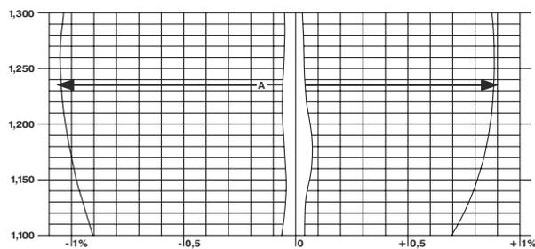
The accuracy of the HYDROVOLT system is further based on the narrow tolerances of the injectionmolded parts. Glass laboratory hydrometers are accurate at their particular reference temperature, but the small hydrometers used in conventional battery testers have - in addition to temperature error - reading errors of up to 2% of the density. These errors result from variations in the size and weight of the component parts due to the
