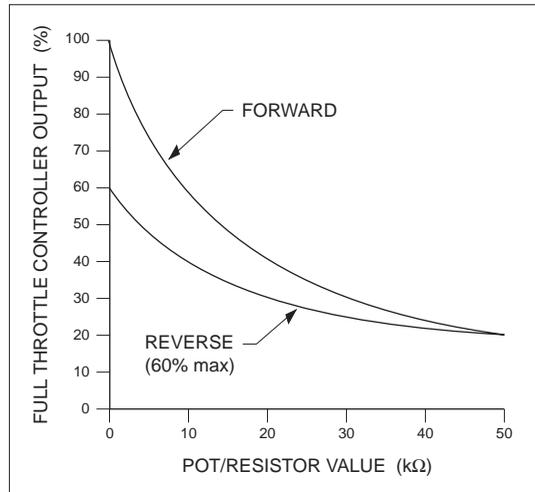
continuous adjustment of the output range down to 20%. It can be used to experimentally “dial in” the desired vehicle maximum speed and then be replaced by a fixed value resistor.
