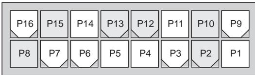
The mating connector is Molex Mini-Fit Jr., part number (5557) 39-01-2165. Contact Molex for information regarding compatible pins for various wire sizes.
