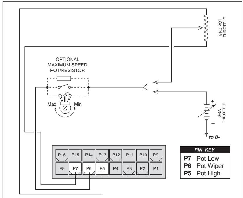
A switch allows the speed limiting pot/resistor to be bypassed if a high speed mode is desired. This switch, which is often called a “rabbit switch,” allows faster speeds for long distance, straight-line traveling.
