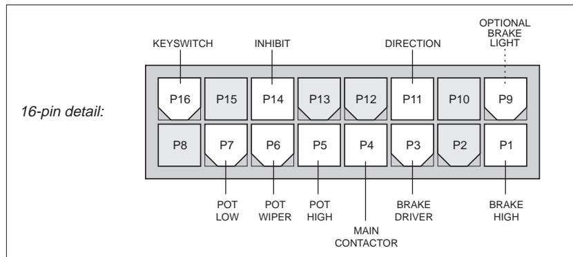
designed specifically for single-ended or for wigwag potentiometer throttles, as well as for several other types of throttles.
