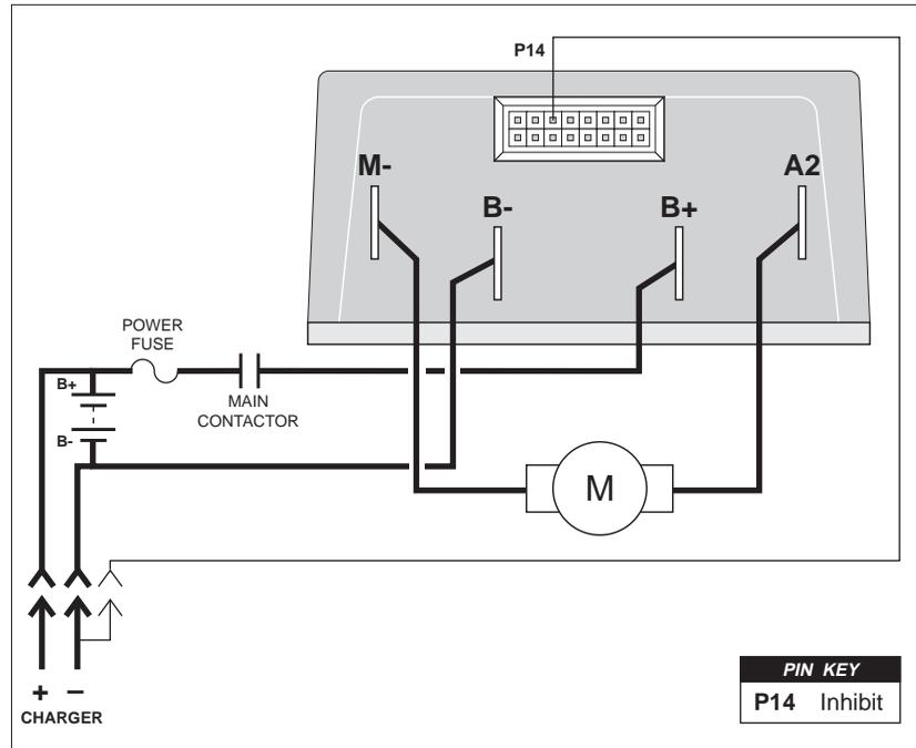
Brake Output / Anti-Roll-Forward, Anti-Rollback
