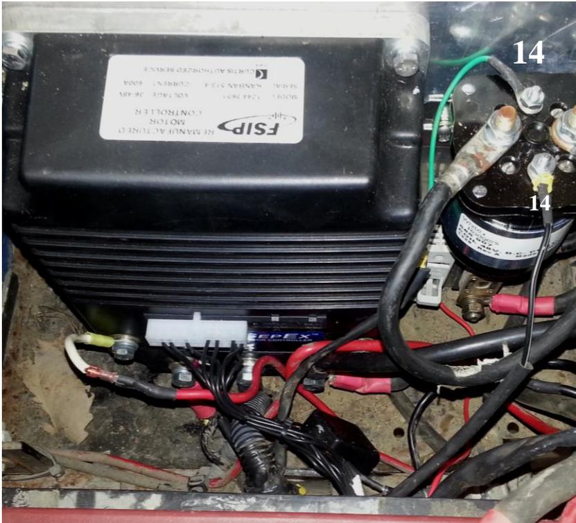
12. Reconnect the motor A1 wire to the B+ terminal of the controller and the A2 wire to the M-. (**Avoid placing wiring in the NCZ-no cable zone**)
