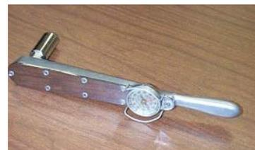
Calibrated torque wrench for hardware installation
