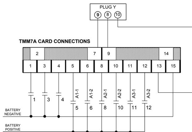
**Section 5.4.2 Typical Brush Wear Sensor Connections**
