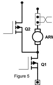
Slow down is accomplished when reversing direction by providing a small amount of retarding torque for deceleration. If the vehicle is moving, and the directional lever is moved from one direction to the other, the regen signal is initiated. Once the regen signal has been initiated, the field current is increased (armature circuit shown in Figure 5). Armature current is
