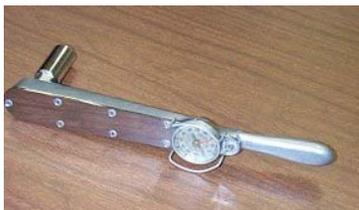
Calibrated torque wrench for hardware installation
