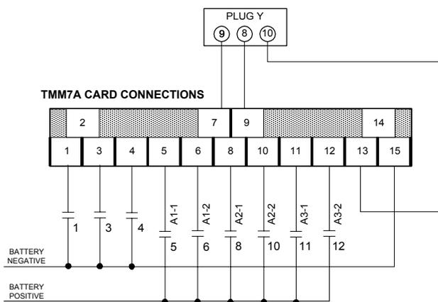
**Section 5.4.2 Typical Brush Wear Sensor Connections**
