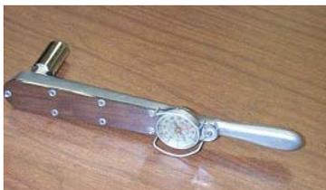
Calibrated torque wrench for hardware installation
