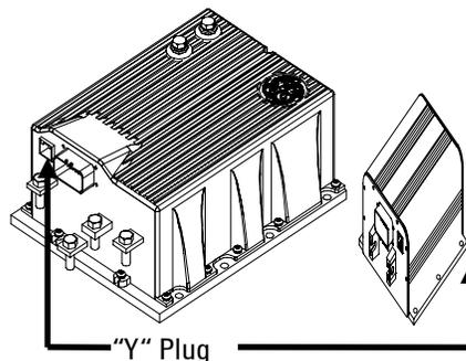
**Handset Cable Part Number - 328A1550ATP1 (12 pin plug)**
