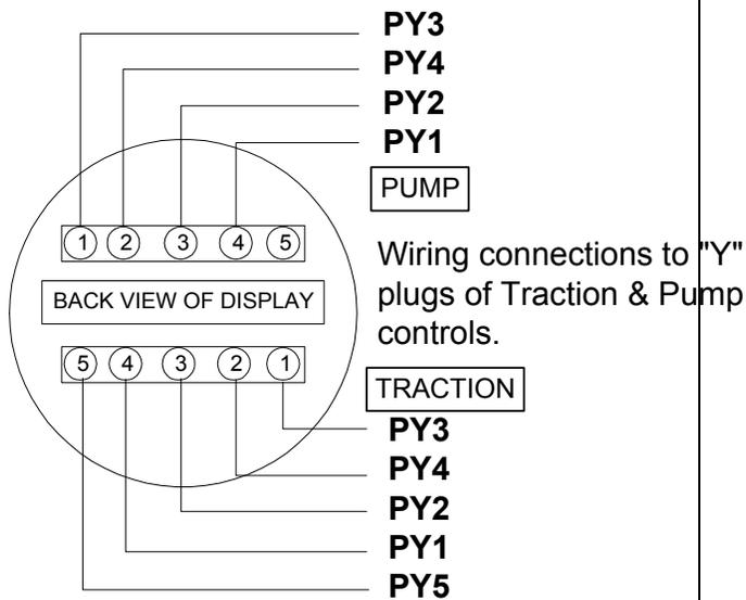
**Section 6.5 Suggested Wiring Configuration for Use of GE Standard Traction/Pump Dash Display with Dual Motor Traction System**
