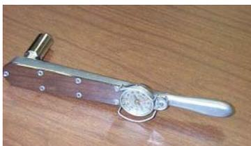
Calibrated torque wrench for hardware installation
