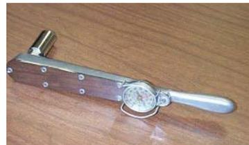
Calibrated torque wrench for hardware installation
