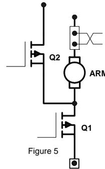
Slow down is accomplished when reversing direction by providing a small amount of retarding torque for deceleration. If the vehicle is moving, and the directional lever is moved from one direction to the other, the regen signal is initiated. Once the regen signal has been initiated, the field current is increased (armature circuit shown in Figure
