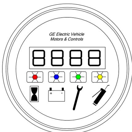
The FSIP Standard Dash Display is a four segment Light Emitting Diode (LED) instrument that displays the FSIP LX, ZX, and SX Status Codes, Hourmeter Readings, Battery Discharge Indication, and Maintenance Required Code. The four LED's above the symbols indicate the active readout mode.
