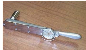
Calibrated torque wrench for hardware installation
