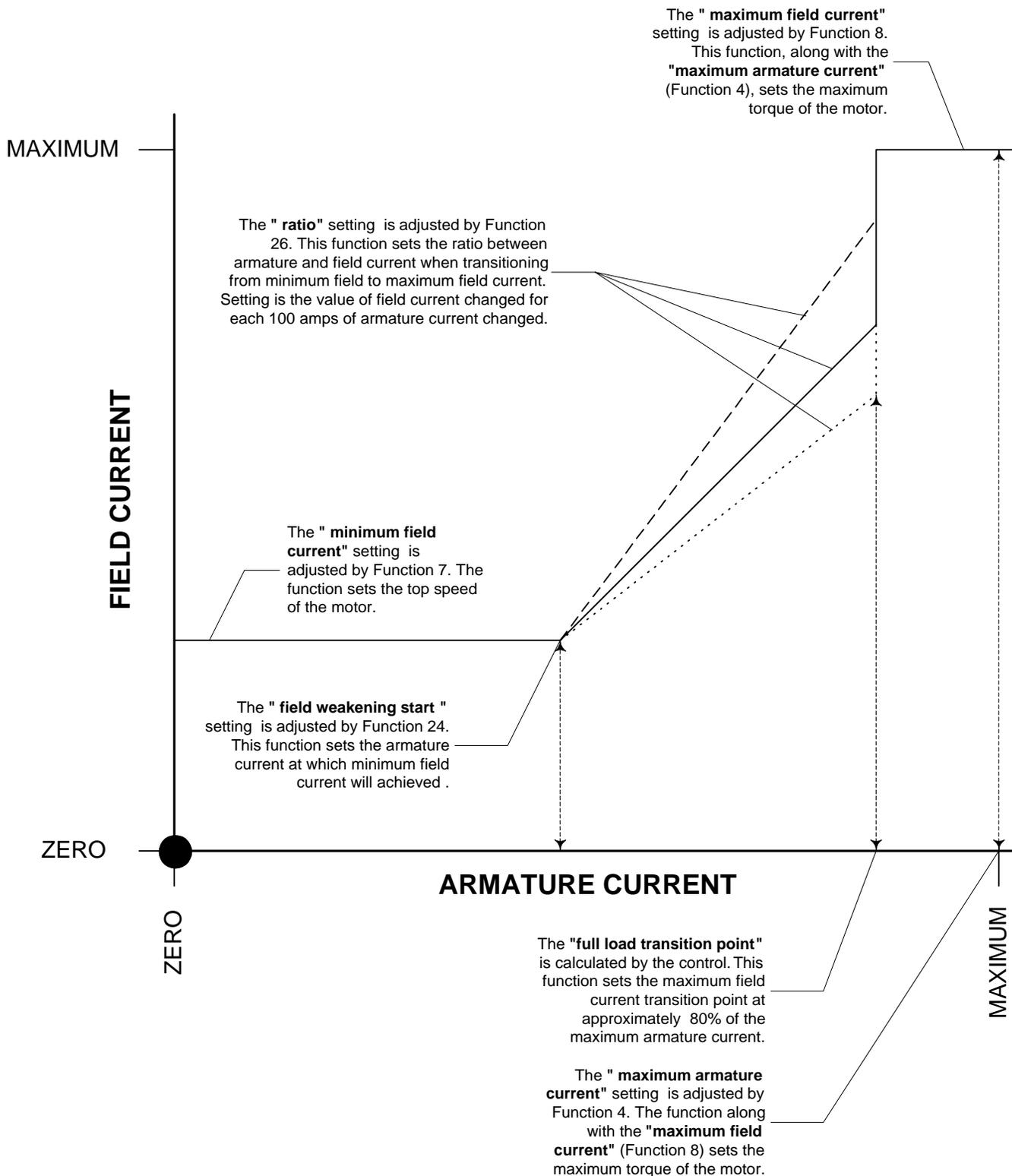
**Section 6.6 Setup Functions for Hydraulic Pump Control**
