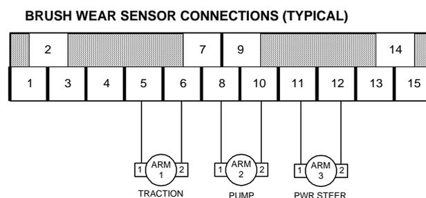
Section 5.4.3 TMM Pump Control Connections
