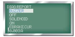
20. SOLENOID: displayed as 'SOLENOID', the next line displays the solenoid state as 'ON' or 'OFF.
