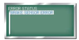
56. Past 7 Error Codes are displayed on ERROR LOG. The error code along with the CPU time (see screen 51) when the error occurred.
