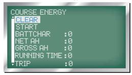
61. Scroll down to 'START' and press the enter key (button 3) to begin recording the energy consumption and begin driving.
