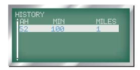
53. TOTAL RUN TIME ON VEHICLE IN MINUTES: displayed as 'MIN', this is the total run time on vehicle in minutes since the last recorded charge cycle.
