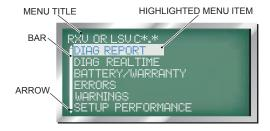
To access the different diagnostic functions, use the five control buttons to scroll through the menus.
