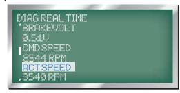
31. MOTOR SPEED SENSOR displayed as 'SPEED SENSOR', displays the status of the speed sensor. For troubleshooting see errors and warning chart.
