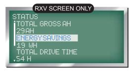
49. TOTAL RUNNING TIME: displayed as 'TOTAL DRIVE TIME', the next line displays the number of hours of running time (pedal down) on the vehicle in hours.
