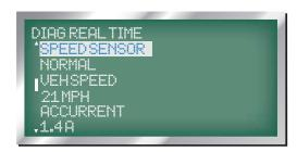
32. MOTOR VEHICLE SPEED displayed as 'VEH-SPEED', shows the actual speed of the vehicle in miles per hour.
