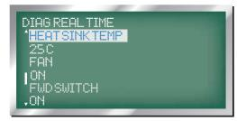
36. FAN function is displayed as "FAN", the next line displays whether or not the controller cooling fan is on or off
