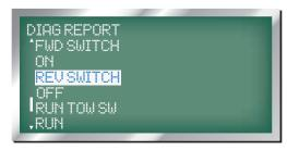
18. RUN TOW SWITCH POSITION: displayed as 'RUN TOW SW', the next line displays the position of the run/tow switch as 'RUN' or 'TOW'.
