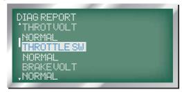
BRAKE SENSOR VOLTAGE: displayed as 'BRAKE-VOLT', the next line displays the sensor voltage as 'LOW', 'NORMAL' or 'HIGH'.
