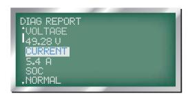
3. STATE OF CHARGE: displayed as 'SOC', the next line displays the state of charge for the battery pack as 'HIGH', 'NORMAL' or 'LOW BATT'.
