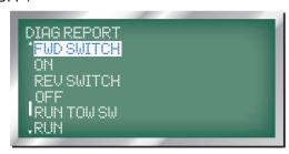
17. REVERSE SWITCH: displayed as 'REV SWITCH', the next line displays the switch position as 'ON' or 'OFF'.
