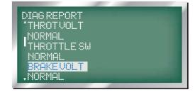
BRAKE SWITCH POSITION: displayed as 'BRAKE SW' the next line displays the switch voltage as 'NOR-MAL' or 'ABNORMAL'.
