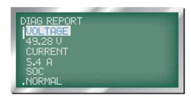
CALCULATED BATTERY CURRENT: displayed as 'CURRENT', the next line displays calculated current as 'HIGH', 'LOW' or the actual number in DC Amps.
