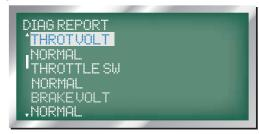
THROTTLE SWITCH POSITION: displayed as 'THROTTLESW', the next line displays the switch voltage as 'NORMAL' or 'ABNORMAL'.
