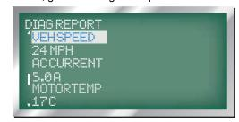
12. MOTOR CURRENT: displayed as 'AC CURRENT', the next line displays the AC current in Amps.
