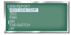
15. FAN function is displayed as "FAN", the next line displays whether or not the controller cooling fan is on or off.
