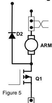
Slow down is accomplished when releasing accelerator pedal or depressing brake pedal by providing a regulated amount of retarding torque for deceleration. If the vehicle is moving, and the accelerator pedal is released, the regen signal is initiated. Once the regen signal has been initiated, the field current is increased (armature circuit shown in Figure 5). Armature current is regulated to the regen current limit as set by Function 9. As the vehicle
