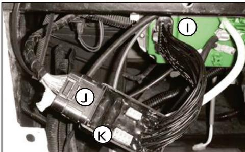
NOTE: The Harness should be oriented and secured with ZipTies so that water and debris does not accumulate in the Connectors.
