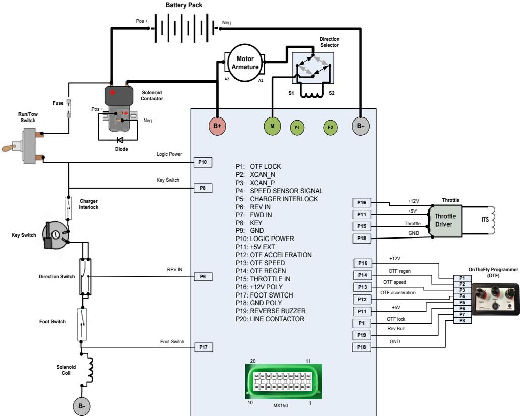
**Navitas TSX3.0 shunt motor controller
