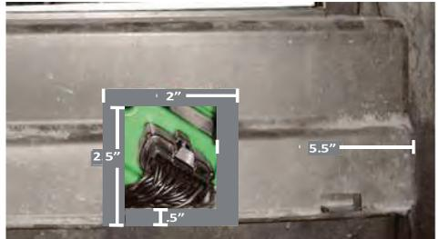
If the Precedent has a six 8V Battery layout, the plastic on the Controller/Wiring Cover may need to be cut out to allow the 20 pin Connector on the Vehicle Module Harness to fit properly.
