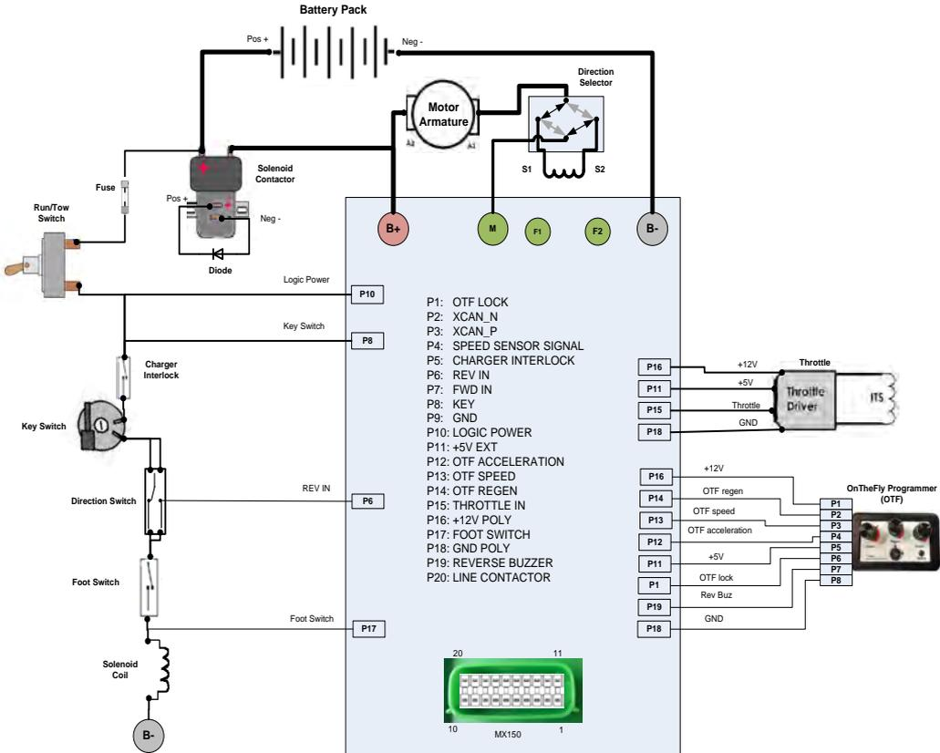
**Navitas TSX3.0 shunt motor controller
