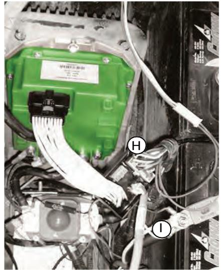
Now the Vehicle's Main Battery Positive and Negative Cables can be re-connected to Battery Pack.
