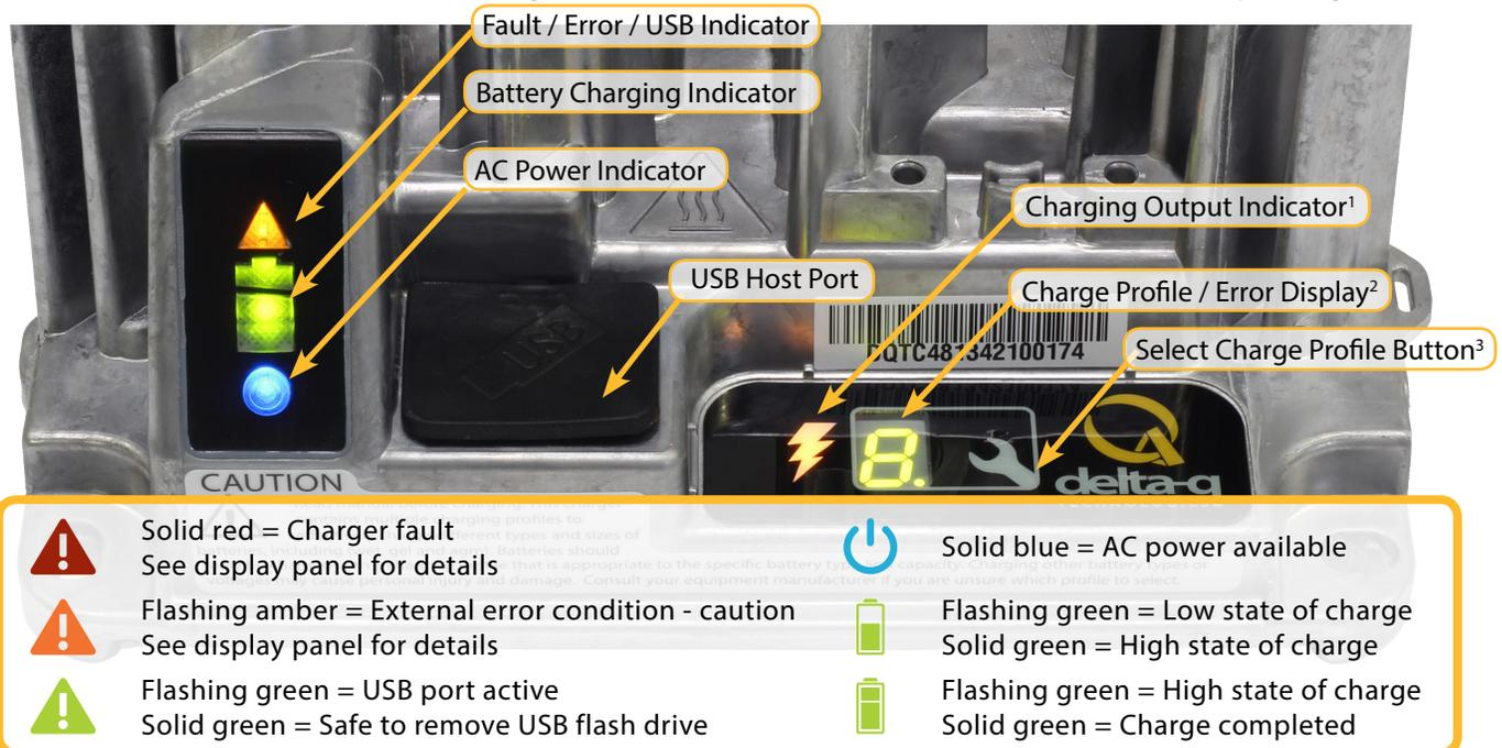
1. The USB Host Port allows data to be transferred to and from the charger using a standard USB flash drive, including the downloading of charge tracking data and updating of the charger's software and / or charge profiles.
