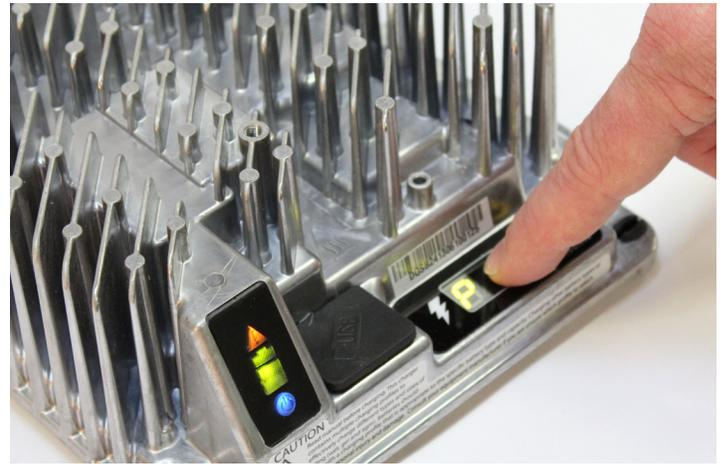
3. Press and release the Select Charge Profile Button to advance through the charge profiles. The selected charging profile will be displayed up to three times (e.g. "P-0-1-1" for Profile 11).\*
