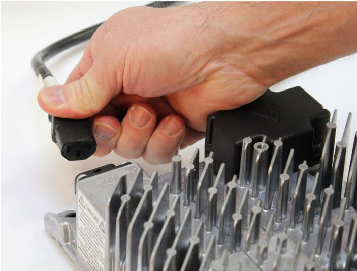
1. Disconnect AC input from the charger, or from the wall outlet. Wait 30 seconds for the input relay to open.
