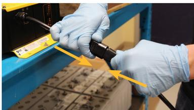
Figure 3: Reconnect AC power to the charger.
