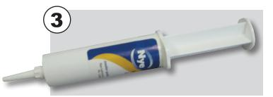
Apply lubricant to each terminal. Reconnect plugs. \*Apply enough lubricant to each terminal opening to completely fill each opening to a depth of .125" minimum.
