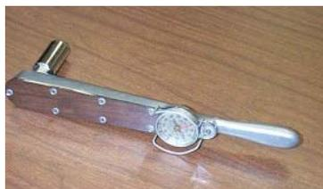
Calibrated torque wrench for hardware installation
