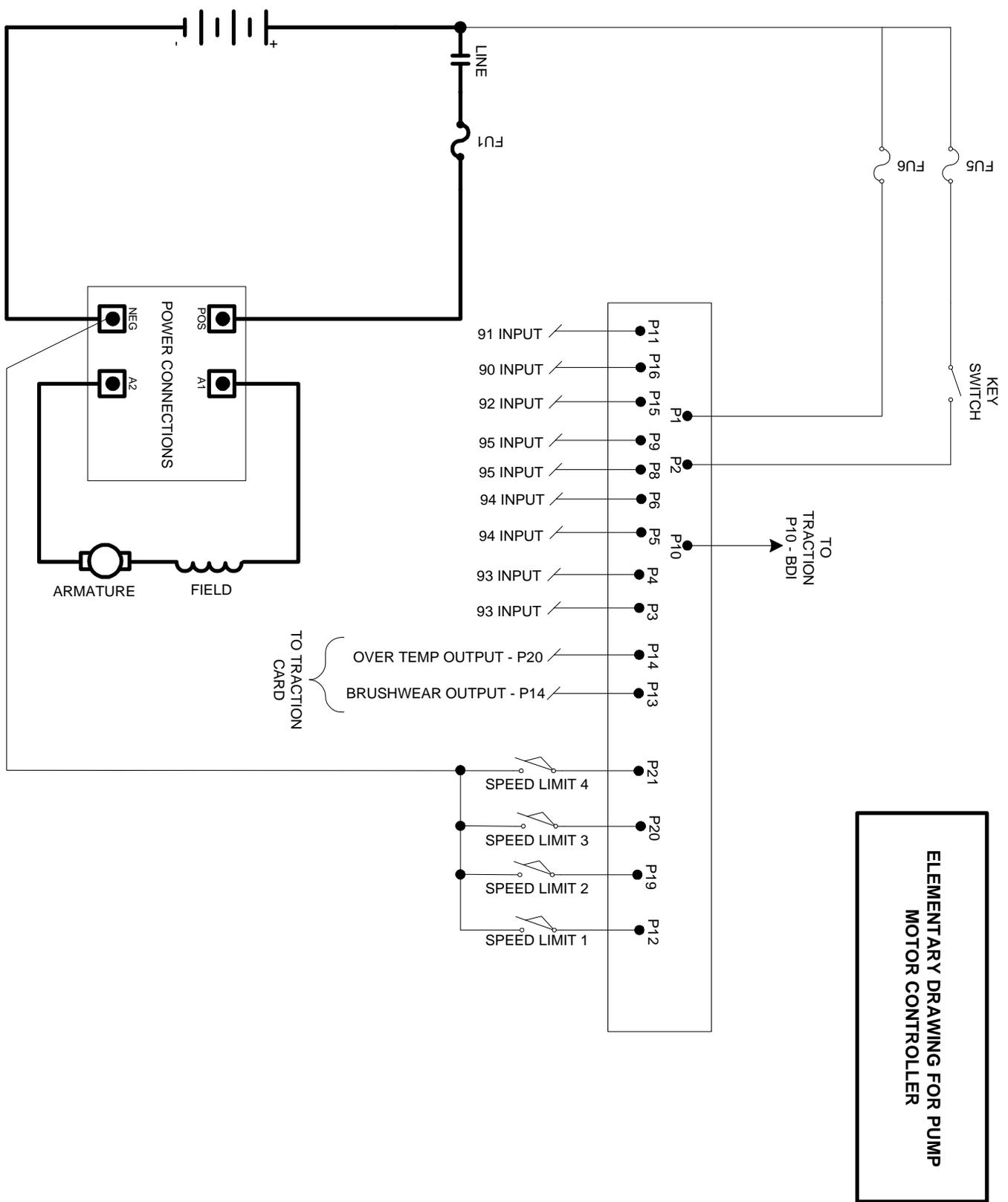
**Section 3.6 Dual Motor Proportioning Drive and Pump Control Input and Output List**
